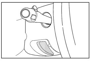
The tilt lever is located on the lower left side of the steering column.
